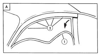
**GB** FIG A. Loosen the rubber door seal (1) in the corner, by pulling it gently from the vehicle. Do not detach it completely.
